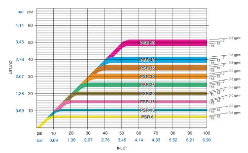
Refer to the performance chart above for maximum recommended inlet pressure for each model. Go to www.senninger.com for larger version; click on "Literature;" click on "Pressure Regulators."
