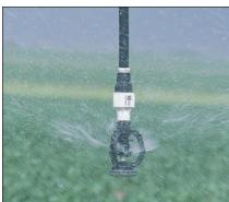
Used for center pivot and other mechanicalmove systems and can be installed at the top of the drop or near the applicator.
